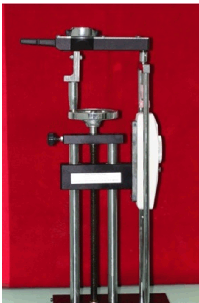
Figure 3: Test assembly, dynamometer and torque meter.
